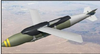
A winged version of the Boeing Joint Direct Attack Munition (JDAM) that will triple the weapon’s glide range to more than 40 miles is a step closer to production after completing wind tunnel tests at a US facility in June.
