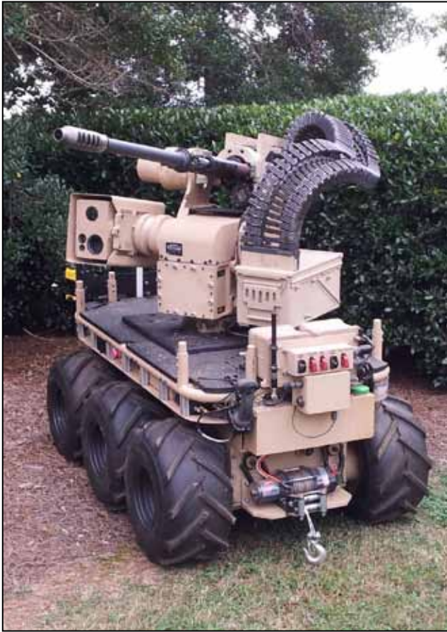
R-400S mounting the ATK M230LF 30 mm cannon. The weapon system is itself mounted on a Northrop Grumman CaMEL military robot.
