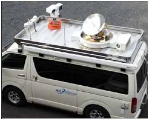
EM Solutions broadband on-the-move terminal atop a communications node being deployed for disaster recovery operations
