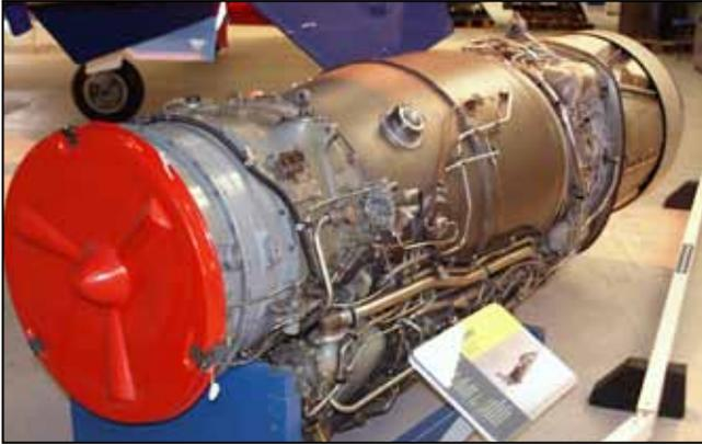
*A F405 engine which is typically used to power the US Navy's T-45.*
