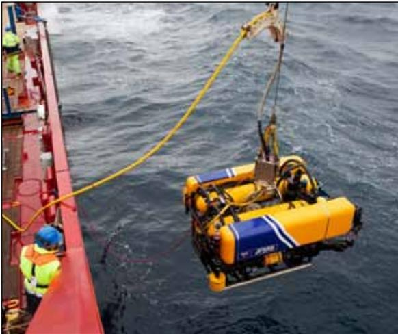
*The ROV (Remotely Operated Vehicle) SC-45 "Scorpio" from James Fisher Submarine Rescue Services is craned outboard from ADV Ocean Shield to locate HMAS Farncomb on the sea floor in the East Australian Exercise Area during Exercise Black Carillon 2013.*
